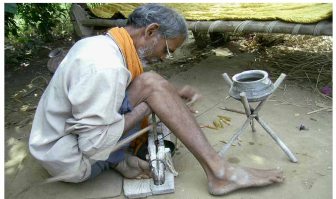
fig. 40. Pratapbhai drilling a bead by placing the bead in a wooden vise bethi
