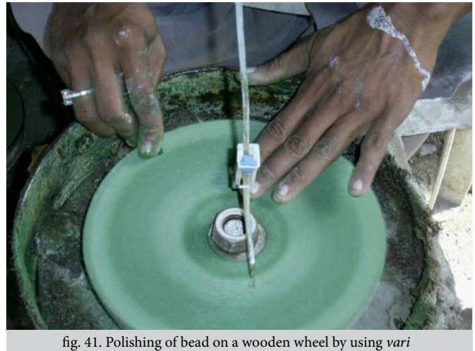
fig. 41. Polishing of bead on a wooden wheel by using vari
